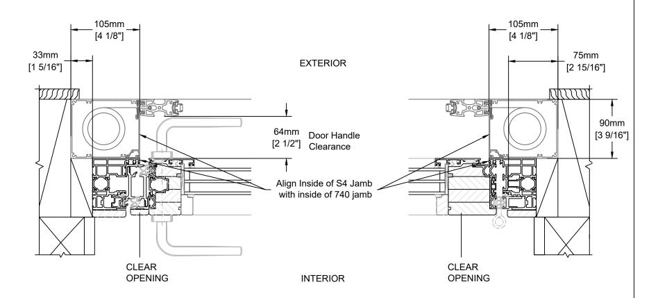
Horizontal Section Jamb with Handle Horizontal Section
