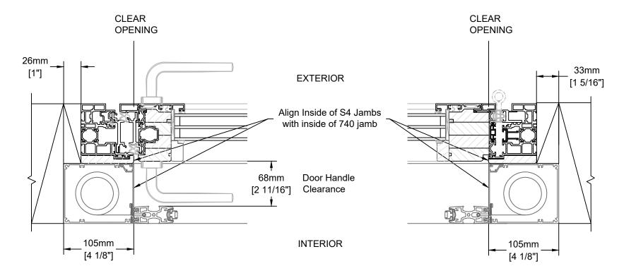
Horizontal Section Jamb with Handle Horizontal Section
